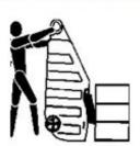
STEP 2: HOLDING ON TO STHE DOLLY, SLIP BOTH LENGTHS OF THE BARREL STRAP OVER DRUM.
